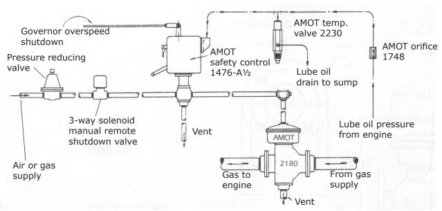
This system will shut down the engine by closing off the gas supply in the event of high water jacket temperature or low oil pressure. Other sensors may be added for overspeed, bearing temperature, compressor interstage pressure, exhaust temperature, crankcase pressure, water pump differential pressure, vibration, and a variety of other parameters.
