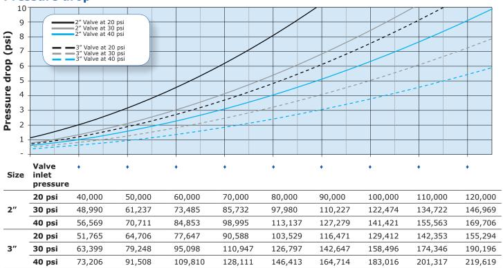
Flow rate (ft³/hr) - Natural Gas at 60°F and 0.65 Specific Gravity
